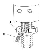
Install the shank washer (1) and locknut (2) onto faucet shank. Tighten locknut securely to prevent collar and spout from rotating. If necessary, support spout base from above to prevent twisting.
